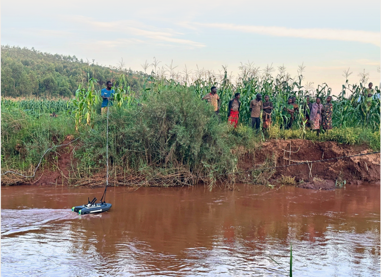
Ariel Nigarura from Université du Burundi uses the Acoustic Doppler Current Profiler (ADCP) to measure the flow of the Waga River, a major tributary of the Ruvyironza.
