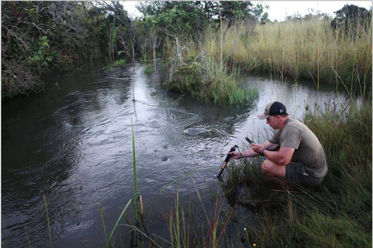
Figure 38. An InSitu Aqua Troll 600 multi-parameter sonde in use on the upper Chambeshi River.
