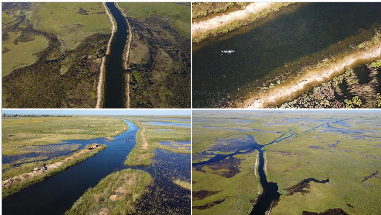
Figure 14. A highway through the swamps — channel dredging in the Bangweulu Swamps improves ease of movement. However, this practice encourages settlement along drainage lines, with the growing population placing resource-use pressure on fisheries and ecosystems in the surrounding catchment.
