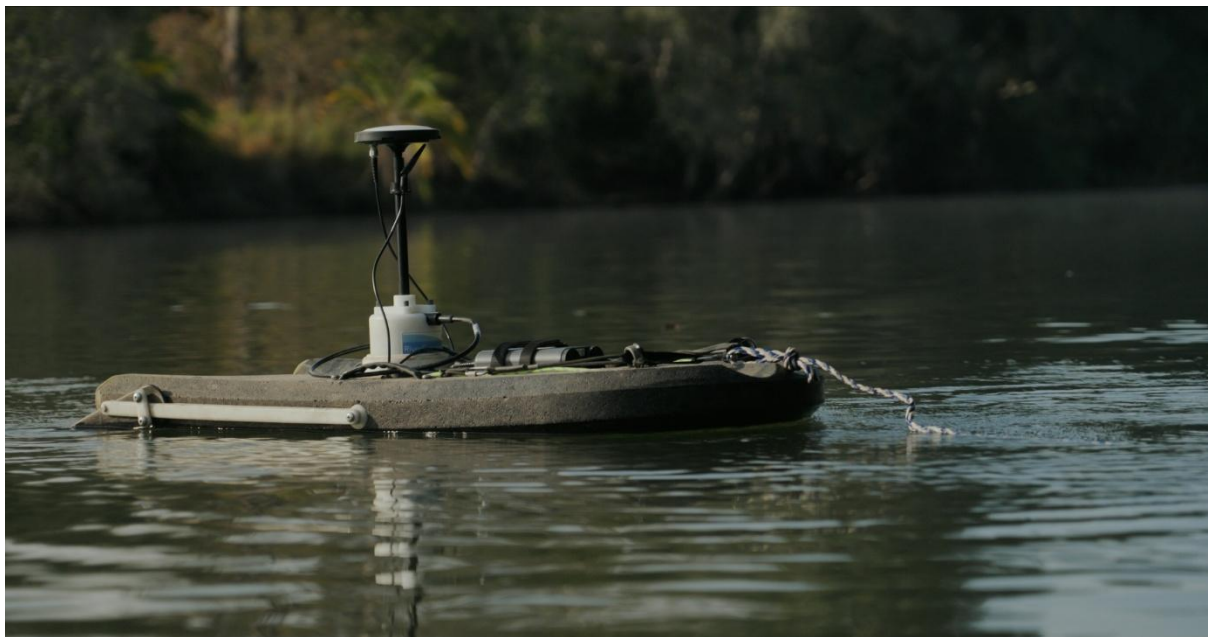
Figure 8. An Acoustic Doppler Current Profiler (ADCP) was used to measure flow, water depth, and channel width at thirteen sites along the transect.
