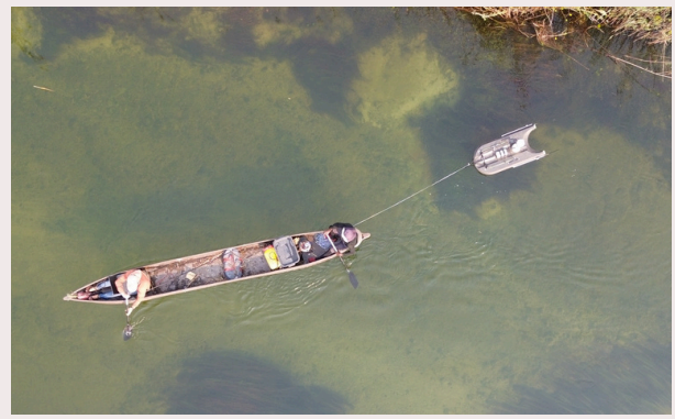
An Acoustic Doppler Current Profiler (ADCP) being towed by canoe. The ADCP is used to collect river flow data.
