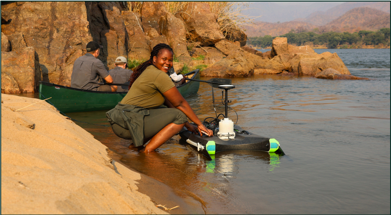
ABOVE: Olivia Marimira from Great Plains assists with deploying the Acoustic Doppler Current Profiler (ADCP). BELOW: This instrument uses sound waves to detect the depth and flow of the river.
