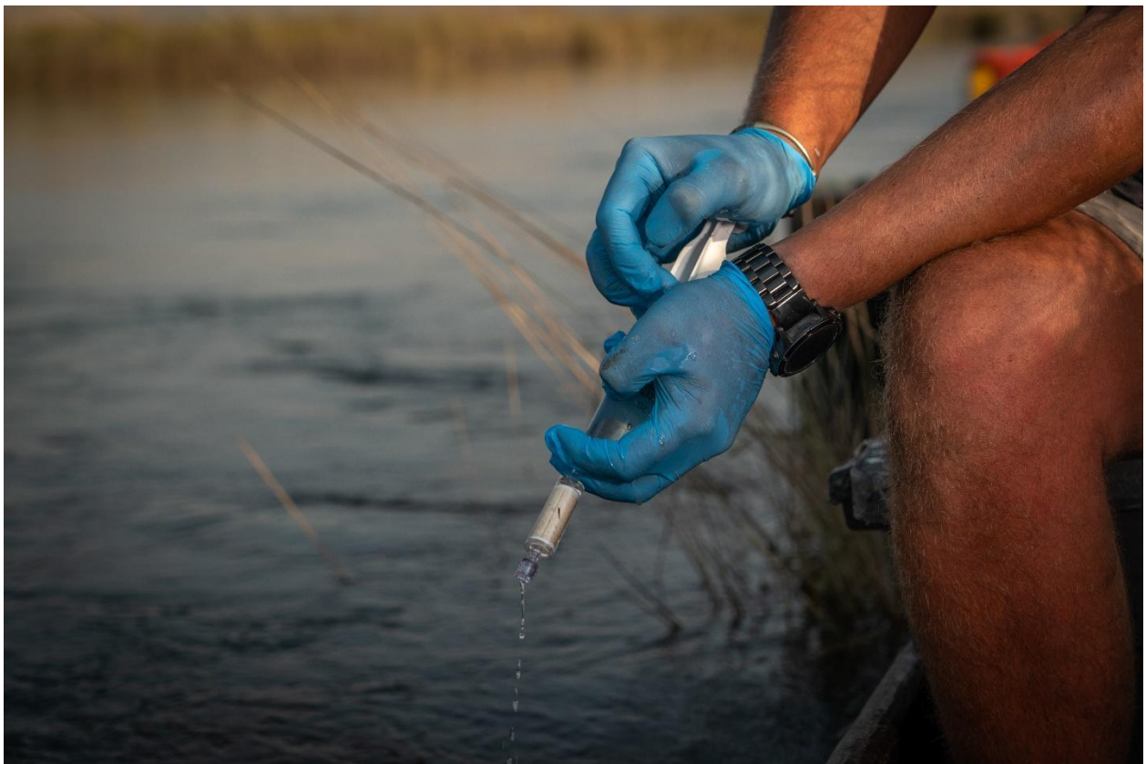
Figure 39. eDNA sample collection using a piston syringe.
