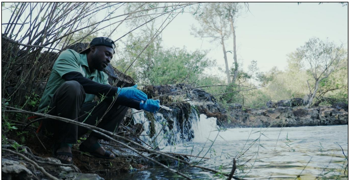
Figure 53: Aquatic eDNA samples were collected by filtering water through a filter.
