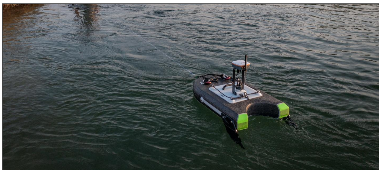
Figure 50: The ADCP used to measure river discharge being towed across the river.
